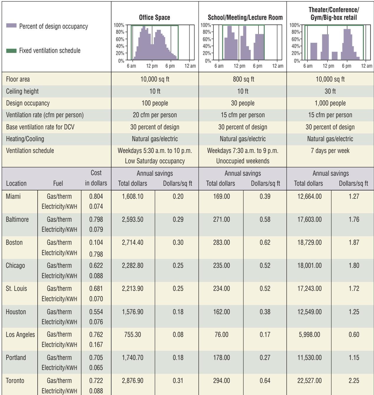
**FIGURE 3. Estimated energy savings for three building types in different U.S. climate zones represented by selected cities. Occupancy densities are different for each building type.**
